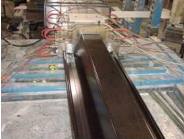
The finished part being pultruded from the die
