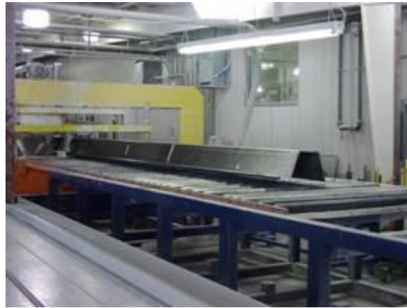
The finished part ready to be sawn to size
